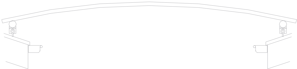
batten awning attached to roof mounted frame
